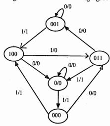
Design the sequential circuit with T flip-flops.
